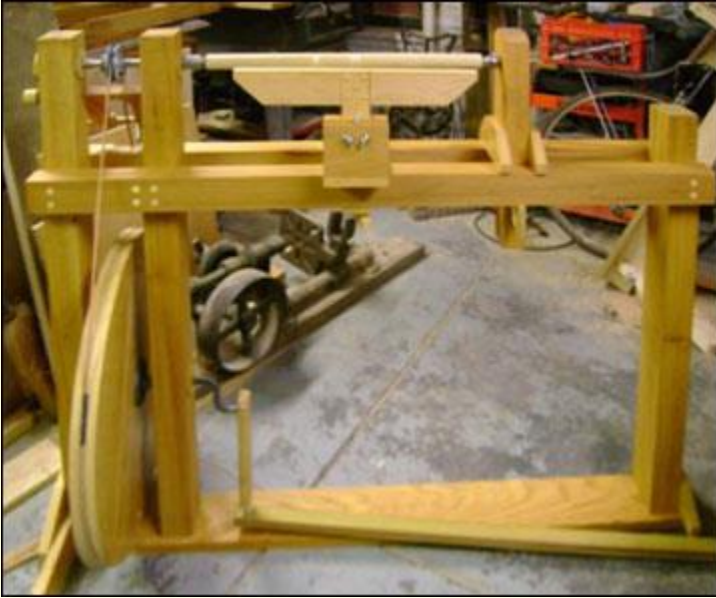
Lathe made by George King. The uprights and lathe bed are from an old piano and other parts (maple) from old library shelving.
