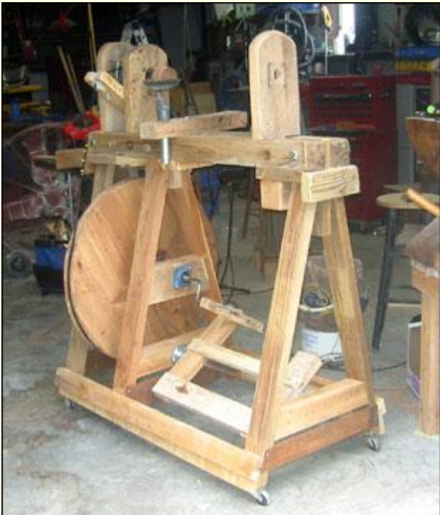
John Webb built this fine lathe mostly from salvaged materials including some 2-1/2" oak from a wrecking yard.
