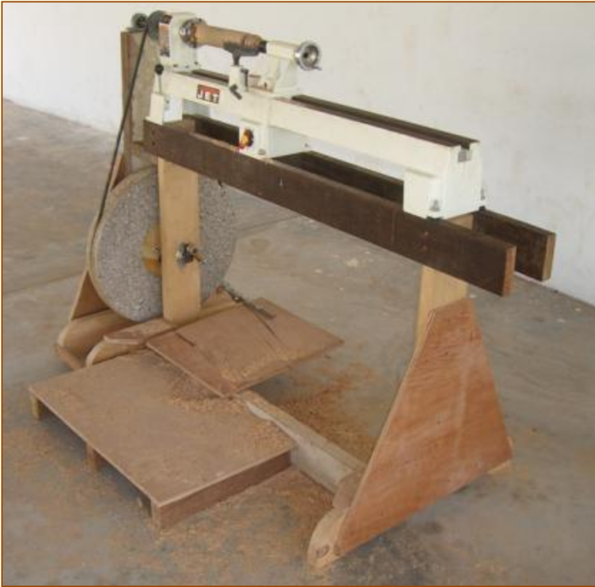
Granite flywheel! This lathe is being used in a mission in Cambodia and is designed to be pumped from the back side by a helper.
