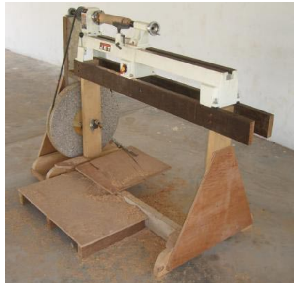
Granite-weighted flywheel! Lathe is being used in a mission in Cambodia and is designed to be pumped from the back side by a helper.
